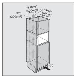
Air intake ① occurs via the plinth at the bottom of the appliance and the air escapes at the top ② at the rear of the surrounding cabinets.
