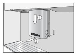
Push the main dispenser down completely ① and remove the stainless steel cover by pulling it off towards you ②.
