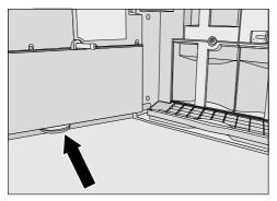
Remove the drip catcher and clean it in the dishwasher or by hand using warm water and liquid dish soap.
