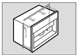
If there is not a seal at the front of the building-in niche, adhere the Miele sealing strips from the back (see picture) before installing the coffee system.The sealing strips can be purchased from Miele.
